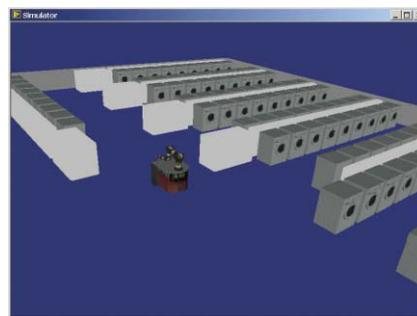
**FIGURE 3.** To allow Mo.Di.Bot to perform tasks autonomously, the washing machine quality-control inspection system was first modeled using Microsoft Robotics Studio and NI's Robotics Simulator.
