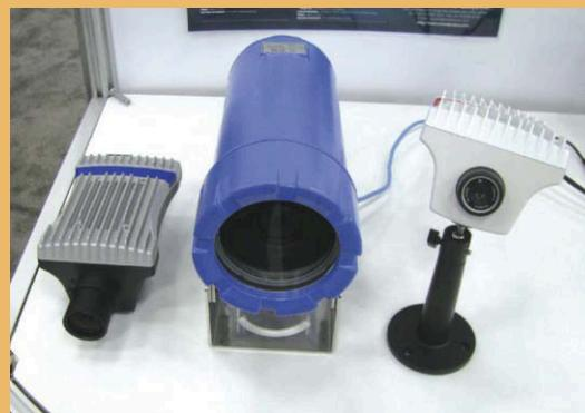
**FIGURE 1.** ORIENT BRAINS' Next-Eye programmable smart cameras use an embedded processor from NI to perform vision tasks. The camera is available in commercial (left), explosion-proof (middle), and IR versions (right).
