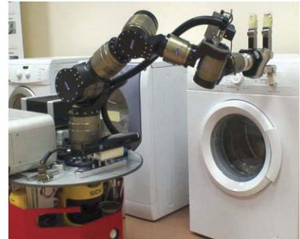
**FIGURE 2.** Mo.Di.Bot emulates many of the functions of a human operator and is capable of autonomously navigating and testing a laboratory replete with multiple washing machines.
