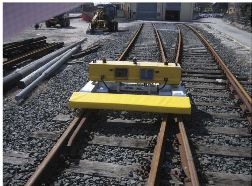
**FIGURE 1.** Felix is an autonomous mobile robot that provides remote inspectors with visual profiles of railroad switches.
